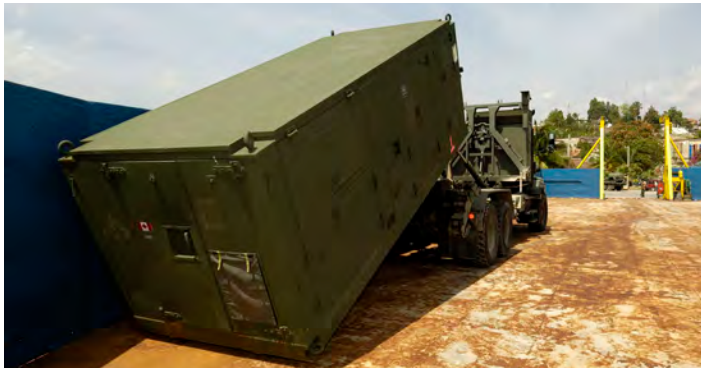
A Heavy Engineer Support Vehicle lowers a ROWPU into position on a barge near Jacmel, Haiti, as part of Operation Hestia in 2010. Photo: MCp David Hardwick
