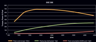
The OXE300 is the most powerful unit in the OXE product line, meeting the demand of users who require high speed and torque capacity for their operations. The twin turbos and the specifically designed gearbox has been developed to withstand the increased torque and power of the 3.0 L aluminum powerhead, providing peak torque at 1750 rpm. Primary customers for the OXE300 are Governmental, Transportation, Search and Rescue and other marine applications with high-speed and load demands.
