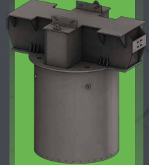
Pile cap design for aggregates jetty
